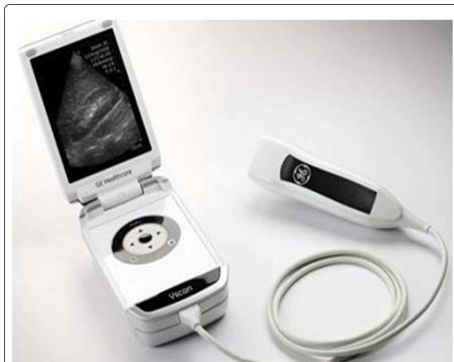
Figure 1: Handheld device used to perform focused cardiac ultrasound.
