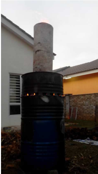
Figure 4. Picture of top Lit Up Draft Furnace
