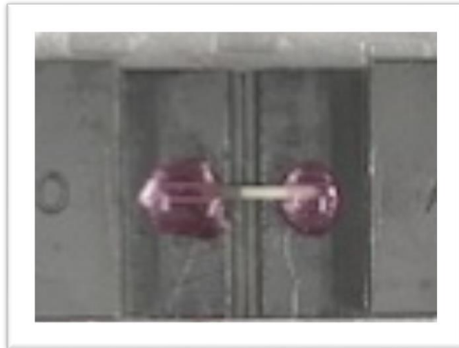
Figure 10. Top view of a composite-dentin beam mounted on a stabilizing jig with cyanoacrylate. Sample is ready to be stressed to failure with a universal testing machine at a crosshead speed of 1 mm/min.
