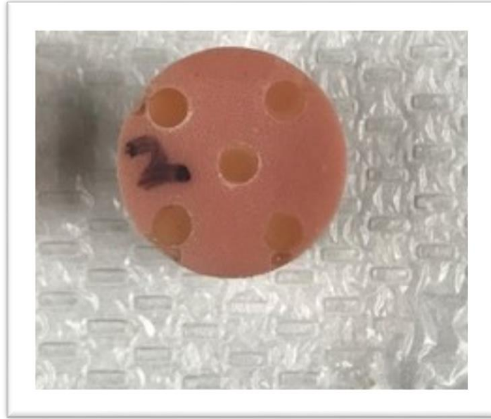
Figure 12. Preparation of specimens for micro-hardness testing. Group 2 (0.1 M) shown above. Five 5 \times 2 mm adhesive discs were embedded to an acrylic mold for testing in the micro-hardness tester.
