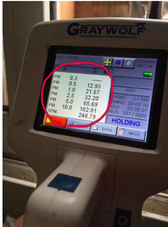
Figure 5: Handheld GrayWolf Laser Particle Counter Model: 3016-IAQ (the data inside the red circle show concentrations of air particulate pollution)
