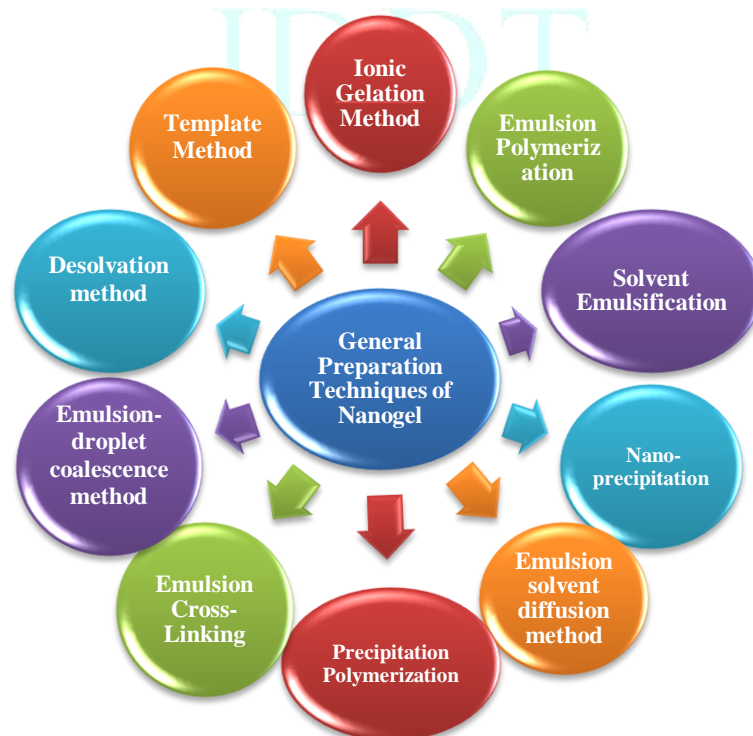
Figure 5: General Preparation Techniques of Nanogel
