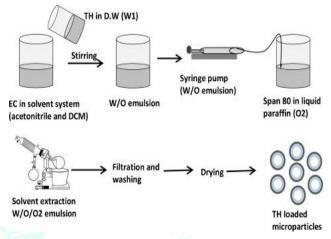
**3. Emulsions Diffusion Method:** In this method encapsulating polymer is dissolved in a partially water miscible solvent and then these solvent is saturated with water. The polymer-water saturated solvent phase is emulsified in an aqueous solution which contain stabilizer, leading to solvent diffusion to the external phase and the formation of nanocapsules or nanospheres.
