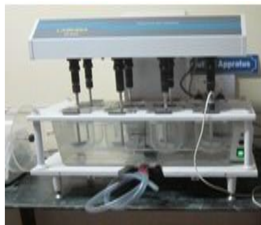
Figure 1: Photographs taken during in-vitro Dissolution study of floating Tablets in 0.1 N HCL.
