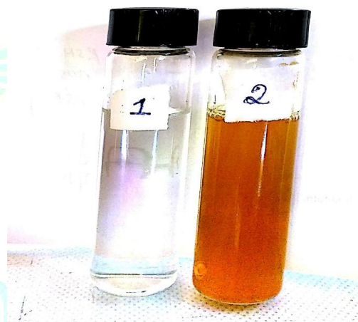
Figure 3.1: 1). 0.01 M Silver nitrate is added to 100mL distilled water, vigorously stirred under 80° C, and 2). After the addition of guava leaf extract.
