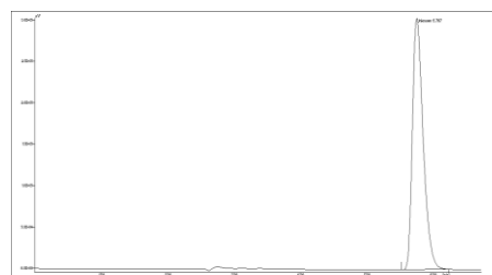
Figure 3: Typical RP- HPLC Chromatogram Brimonidine Tartrate (40 µg/ml) with corresponding retention time.
