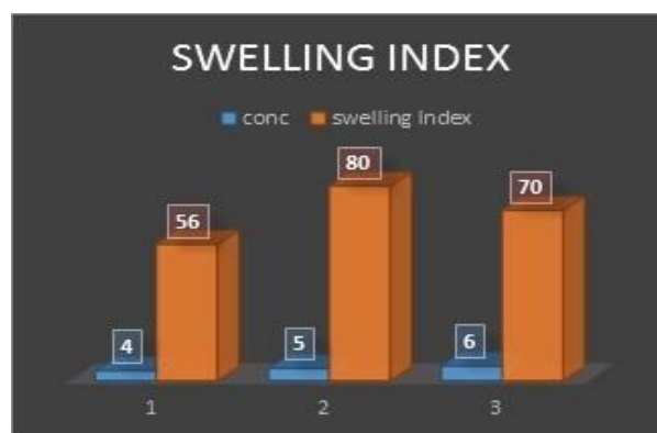
Figure 4: Effect of concentration of polymer on swelling index
