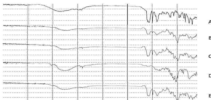
Figure 1b: IR spectrum of A) Drug B) Drug+Sodium Starch Glycolate C) Drug+Cross Camallose Sodium D) Drug+Lactose E) Drug+Microcrystalline Cellulose.
