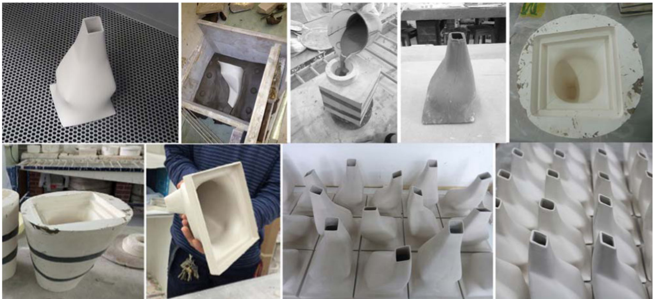
Figure 8. Sinuous Cones production process: 3-d print model, generation of plaster mould, and slip-casting to obtain the final ceramic pieces.
