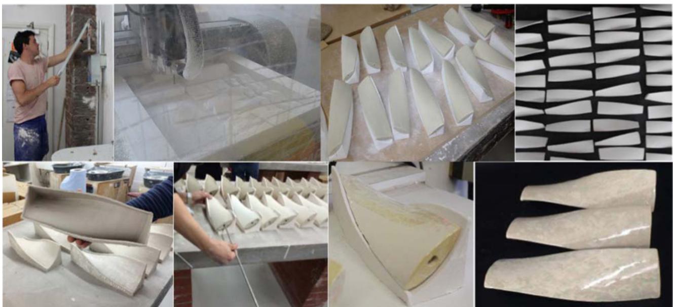
Figure 6. Cruciform Helix Surface: extrusion, components in polystyrene formers, plaster mould for formers and final ceramic formers, and final glazed components.
