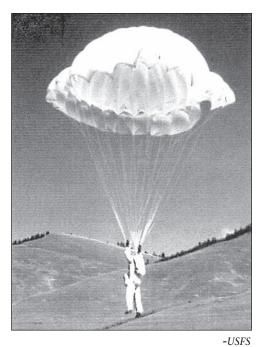
Francis Lufkin making experimental jump to test static line deployed Eagle
