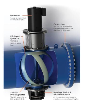
Figure 12: Schematic of a Lucid turbine [68].
