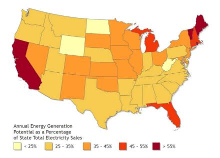
Figure 7: Potential annual generation from rooftop PV on all buildings as a percentage of each state's 2013 total electricity sales. Figure from NREL [44].
