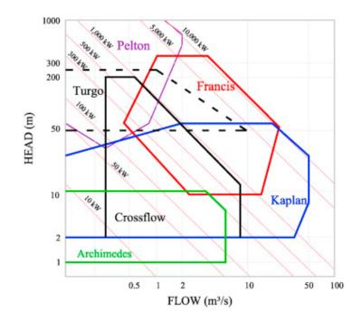
Figure 8: Types of turbines suited to different situations and their expected generation (used with permission) [52].
