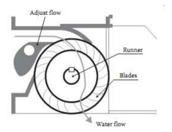
Figure 9: Schematic of a crossflow turbine. (used with permission) [55].
