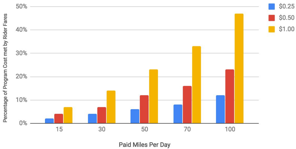
Figure 3: Graph of the percentage of demand-responsive system cost met by rider fares according to each fare option and paid miles per day.
