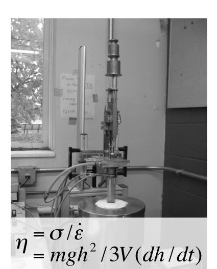
parallel-plate viscometer  $max T = 1100^{\circ}C$ η range 10<sup>9</sup>-10<sup>12</sup> Pa s
