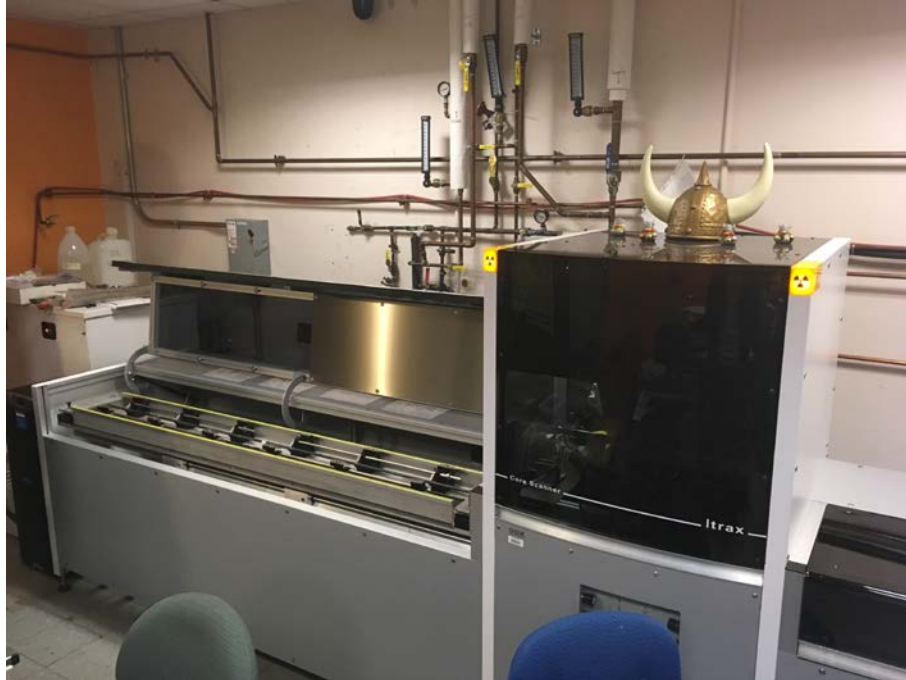
Figure 2.9: The Cox ITRAX XRF Core Scanner at the Ronald B. Gilmore XRF Laboratory at the University of Massachusetts, Amherst.
