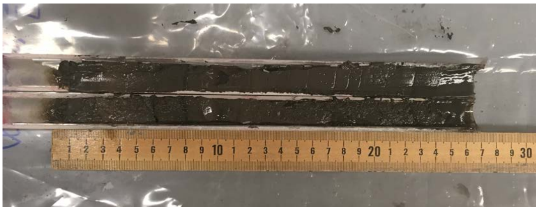
Figure 2.7: The receiving tube from sediment trap C4 after being scored and split.
