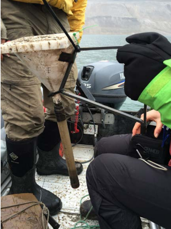
Figure 2.2: A sediment trap after removal from the mooring line
