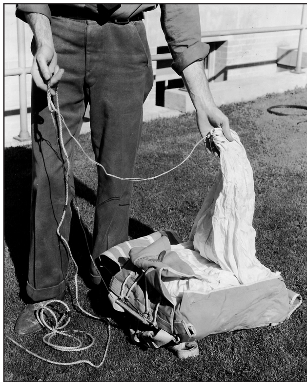
1940 First Static Line: Metal ripcord attached to line running to apex of parachute; rope static line attached to junction of ripcord/line to apex. (Frank Derry collection)
