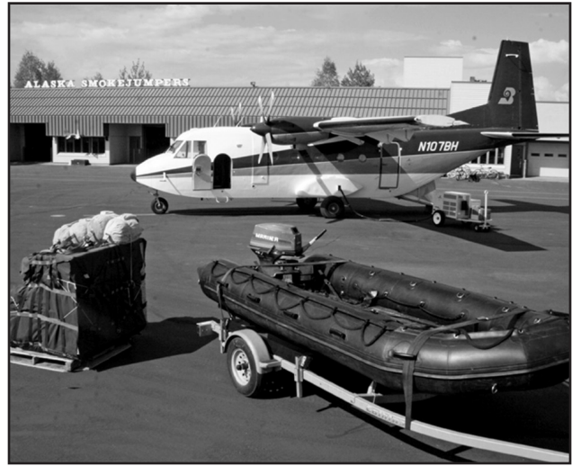
Zodiac on pallet ready for delivery by paracargo, inflated Zodiac with motor. (Courtesy Alaska Smokejumpers)
