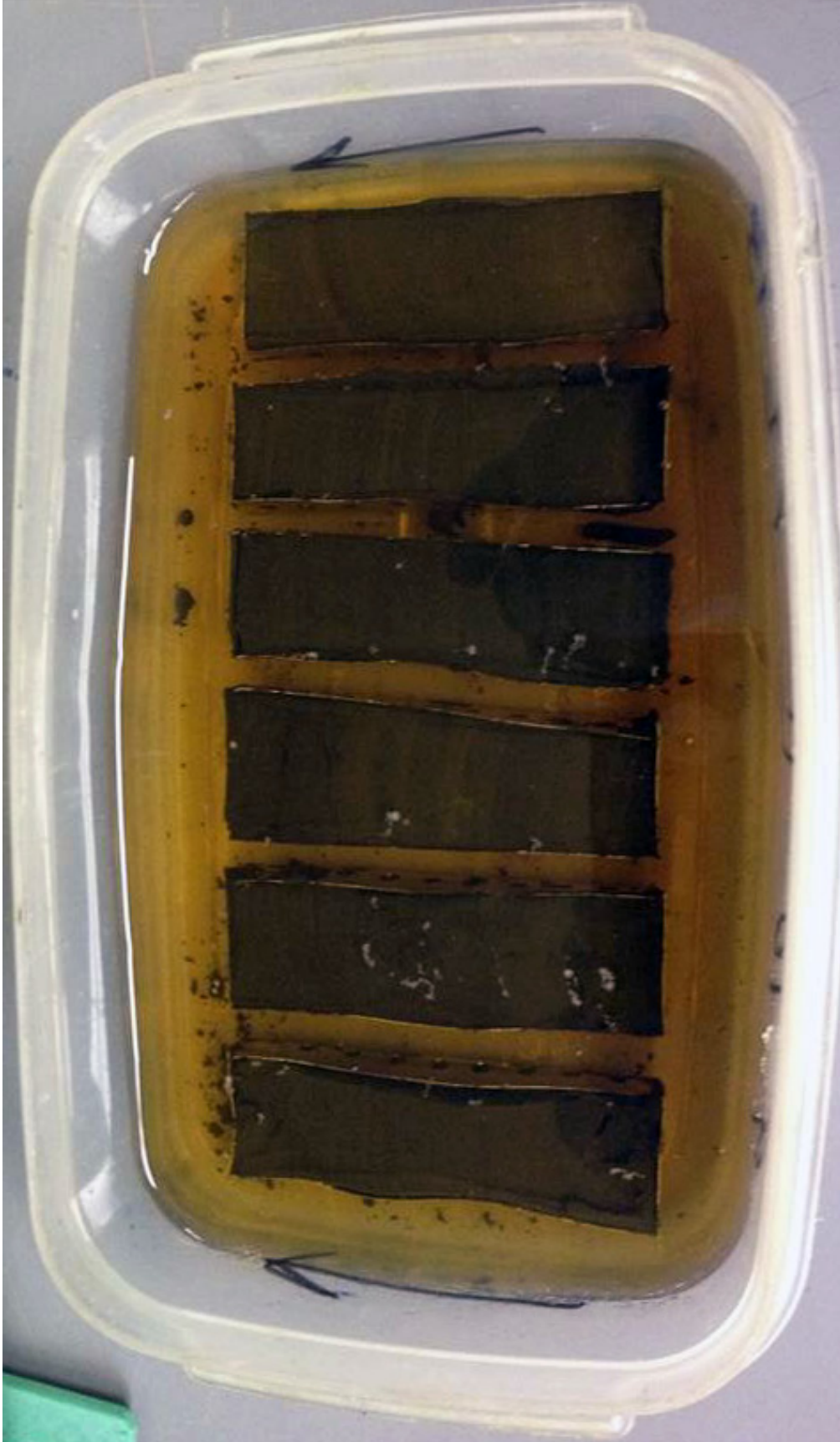
Figure 12 -A photograph of six LH-4 subsamples submerged in their final bath of 100% epoxy. The arrows indicate the upwards direction. The hardened block of thin sections was trimmed with a bandsaw and then sent away to be ground and mounted on slides. All thin sections created overlapped by 1 cm to ensure complete core stratigraphy was included in atleast one thin section.
