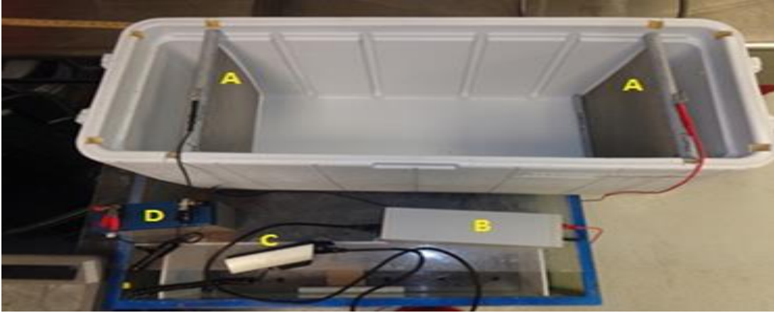
Figure 1-1. Portable LVEA Apparatus as described in text. Consists of cooler, electrodes (A), power supply (B), inverter (C), and battery (D).
