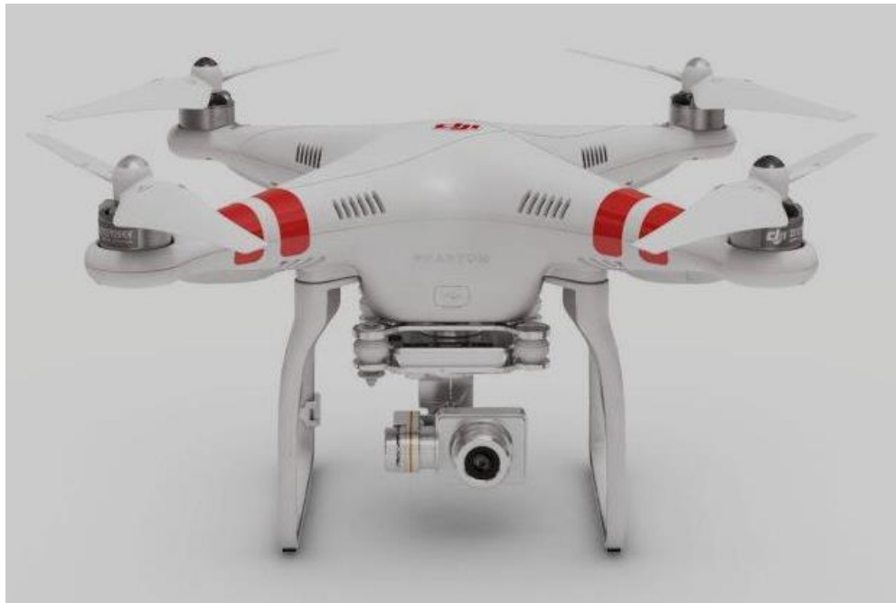
Figure 3 The unmanned helicopter DJI Phantom 2 vision+.
