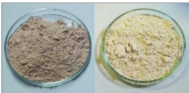
Fig. 1 – Appearance of the powders of Ben (left) and Zeo (right) materials.
