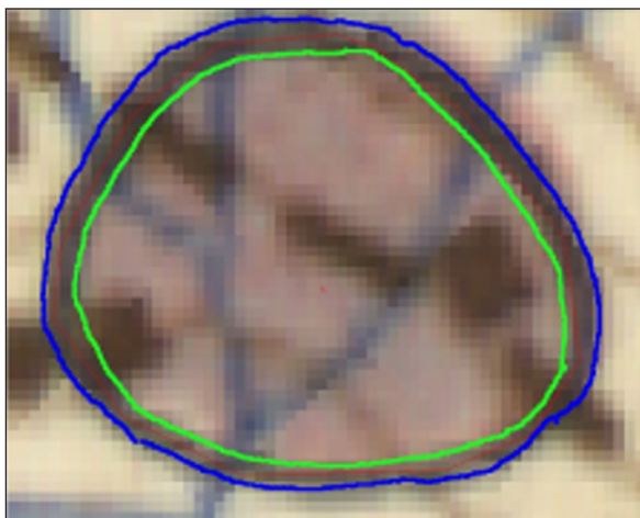
Figure 6 - Variation of an area depending on the location of the digitized boundary with respect to the original line drawing in IKFM, external (blue), intermediate (red) and internal (green) margins of the border are indicated.
