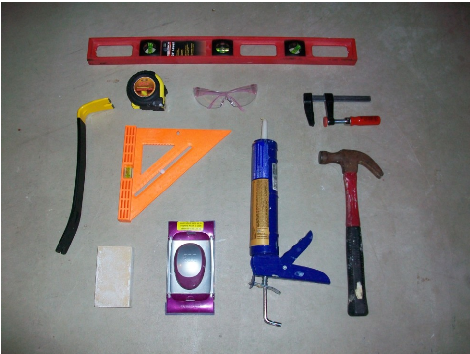
Figure D 4. 24" level, tape measure, crowbar, safety goggles and clamp. Right angle/level, contractors adhesive and dispensing gun, hammer, fine grade sanding block and 3M sandpaper holder
