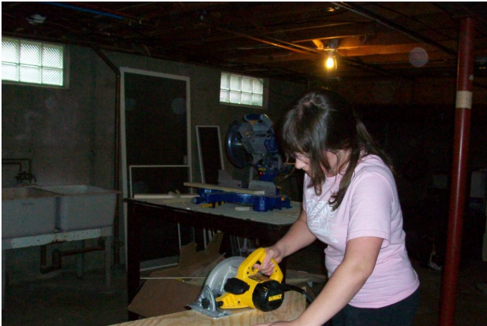
Figure D 10. A lower table for using the circular saw provided good leverage also.
