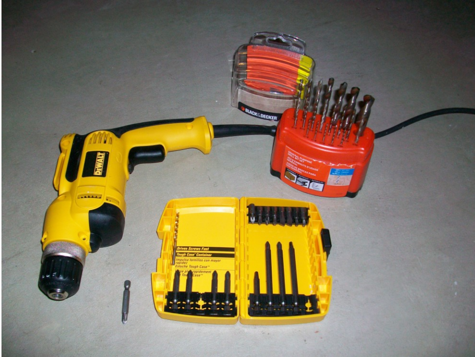
Figure D 5. DeWalt corded screw gun/driver with sets of screw and drill bits
