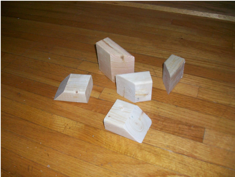
Figure B 15. These are 'brackets' I cut from scrap 2x4s and used to help attach the front piece of plywood to the side panels.
