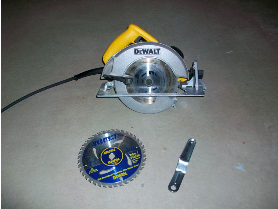
Figure D 1. DeWalt 7 1/4 inch circular saw with two blades; one for rough cuts, one for finishing work
