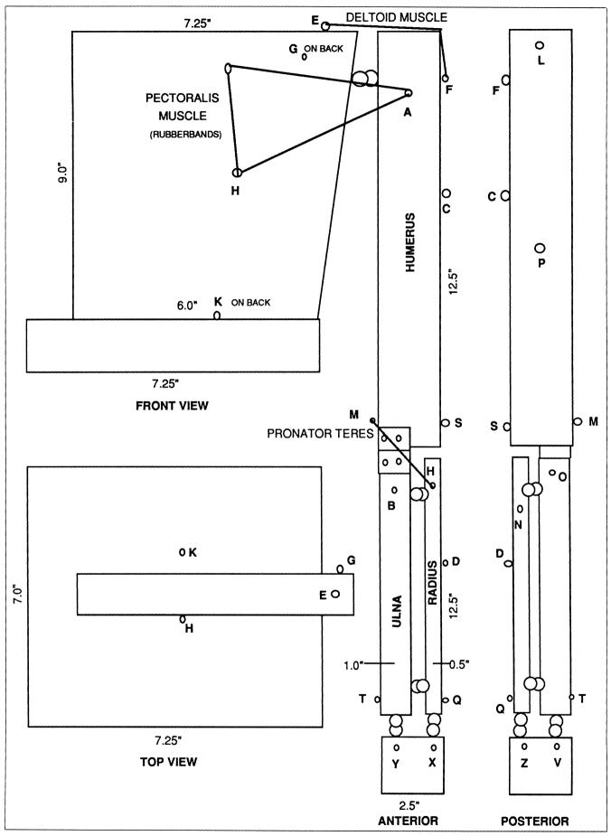
Figure 2. Details for the construction of the musculoskeleton model.
