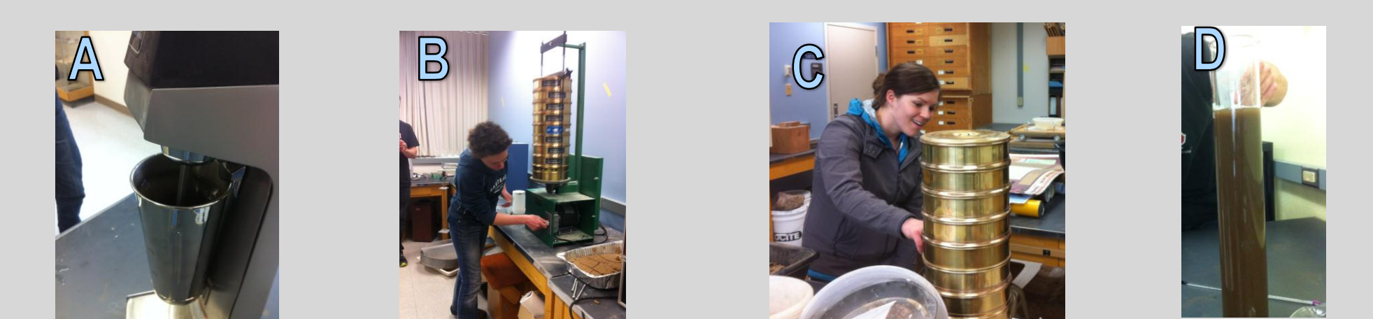
FIG. 9. A. Mixing the sample B. Natasha sets the sieve C. Camie weighs pans D. Hydrometer test
