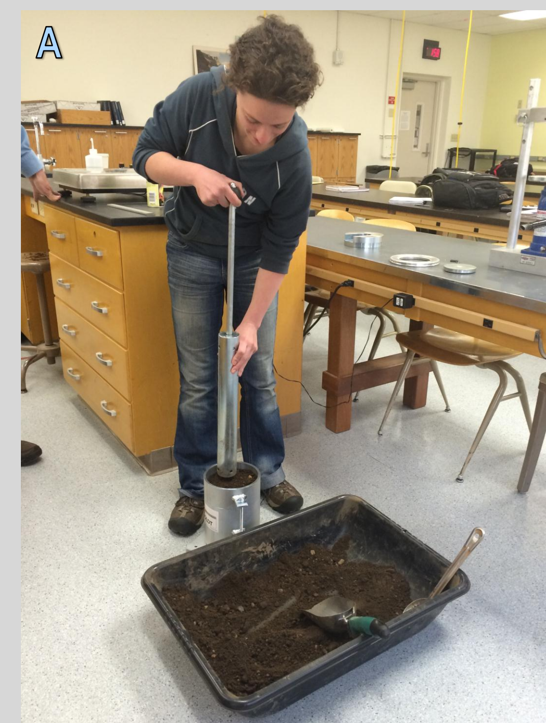
FIG. 7 A. Natasha preparing 1 of 3 lifts
