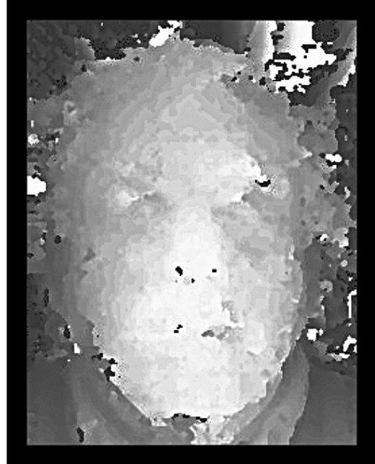
*Figure 7-11 Final depth map after cropping, scaling, equalizing and sharpening*
