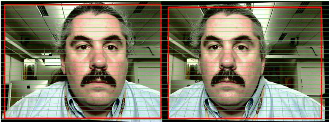
Figure 7-7 is an example of a rectified stereo pair showing the regions of interest and correspondence epilines.
