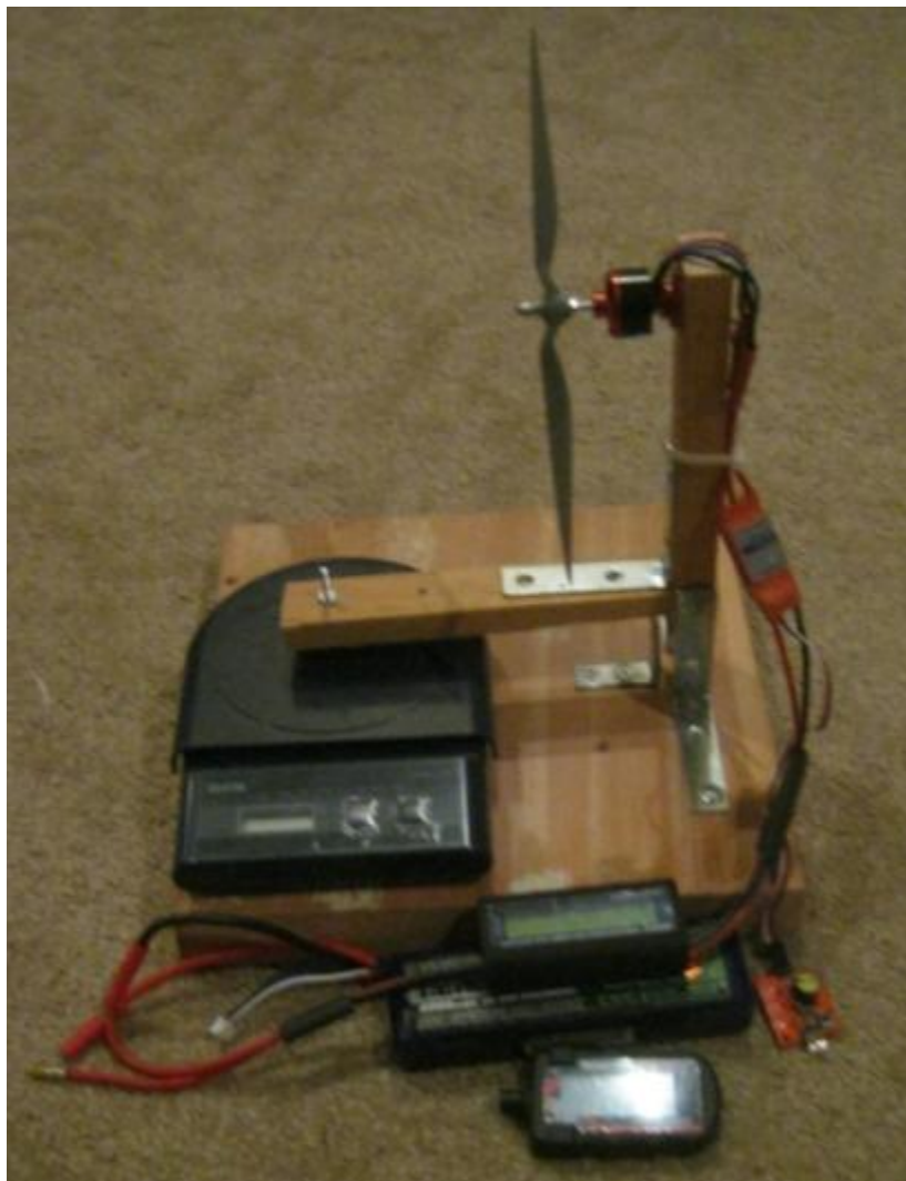
Figure 8: Thrust Measurement Setup
