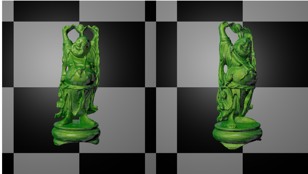
Figure 6: The Stanford Happy Buddha model rendered with out interlacing (left) and with (right) interlacing across two frames
