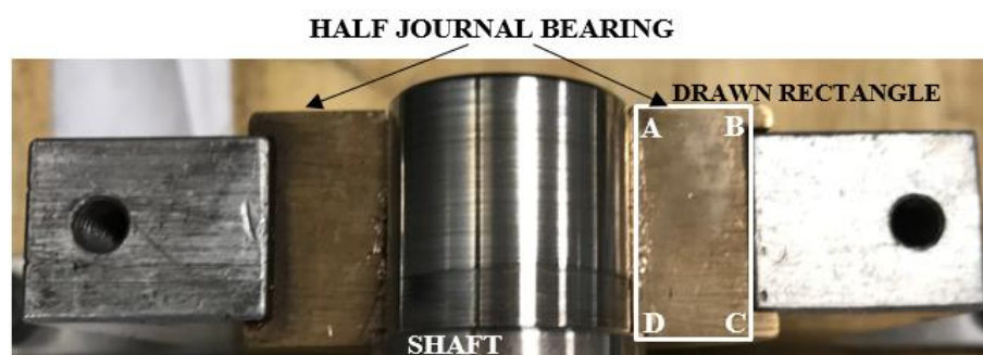
Figure 11: The Half Journal Bearing under Investigation
