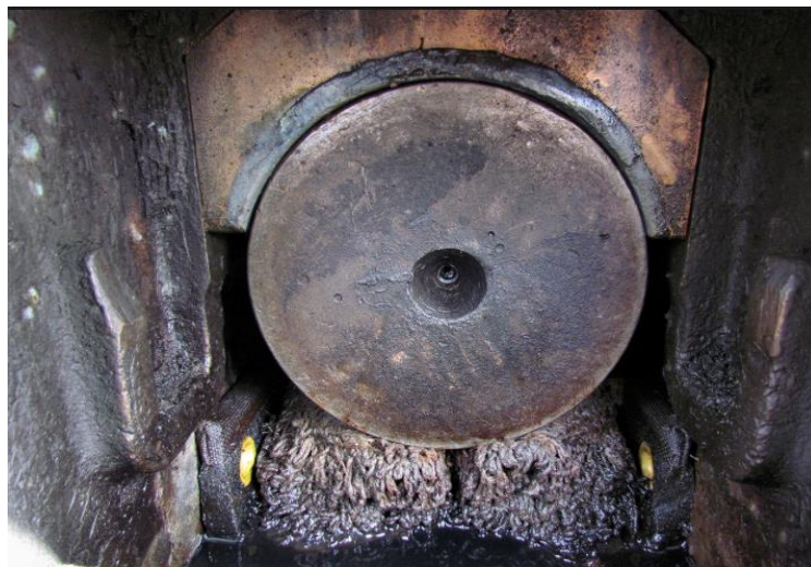
Figure 5: Bearings in Railway Goods Wagons [73]
