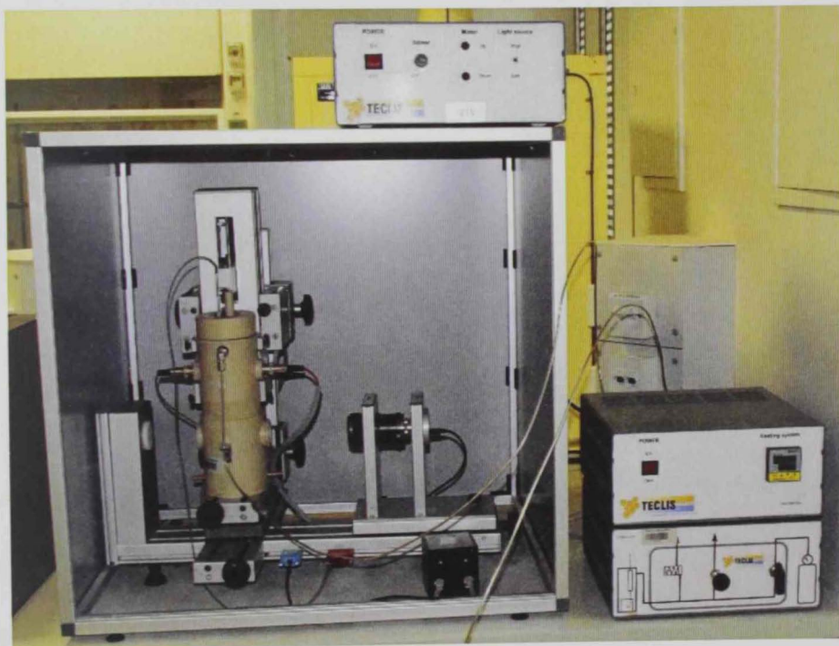
Figure 2.6: Teclis-Tracker used for IFT and contact angle measurements
