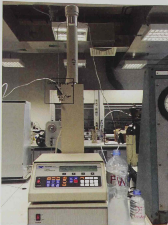
Figure D.3: Injection pump
