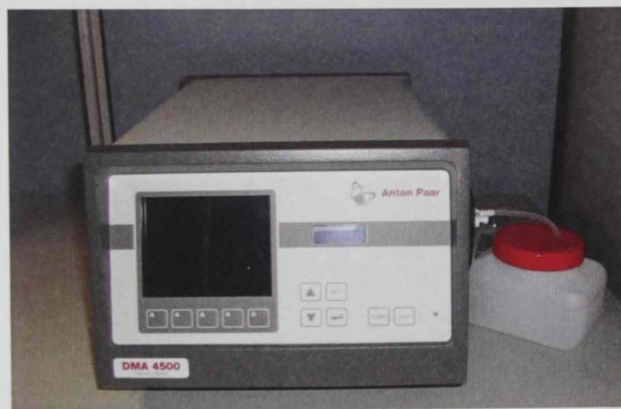
Figure 2.1: HPHT vibrating tube densitometer
