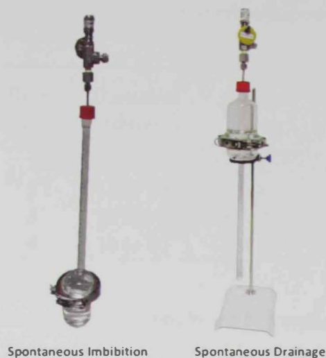
Figure 2.8: High temperature Amott Cells (Vinci Technologies, France)
