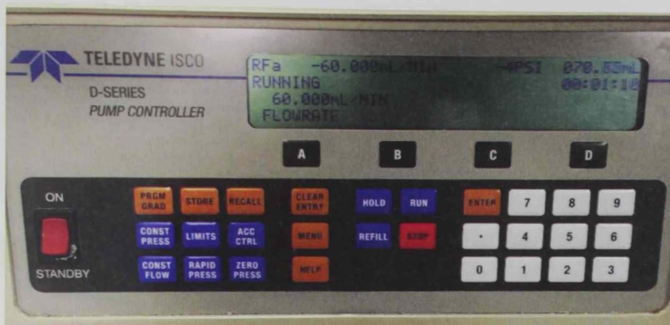
Figure D.4: Pump controller of the injection pump
