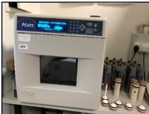
Figure 11: The CEM mars 5 microwave digestion system
