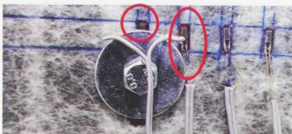
Figure 4.22: Photo of the damaged strain gauges in S\_6D connection between "B2" and "B3"
