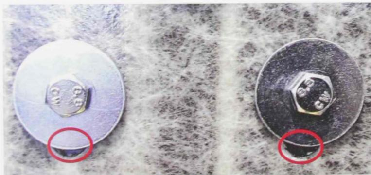
Figure 3.43: Bearing failure of W2\_D10\_ST\_1 connection
