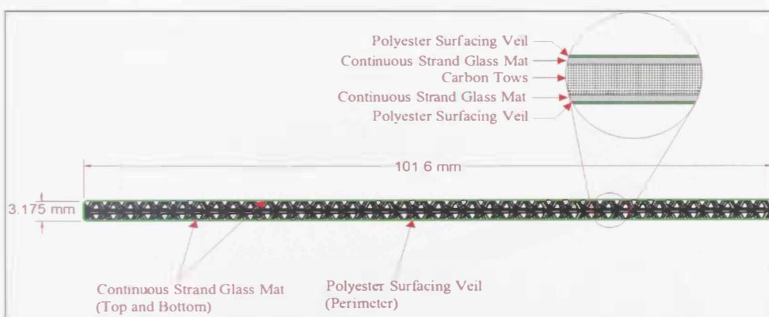
Figure 3.1: Cross-section of the HFRP laminate used in the experimental study
