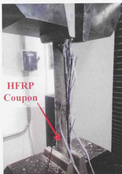
Figure 3.5: Photo of the HFRP coupon after failure
