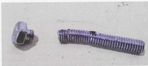
Figure 3.34: Shear failure in the bolts of W2\_D8\_T3\_1
