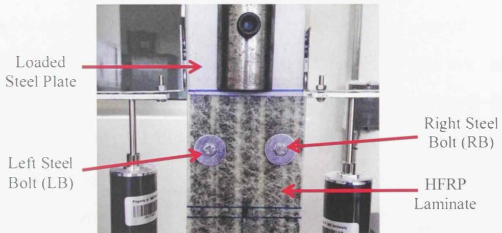
Figure 4.10: Typical locations of steel bolts in the experimental setup of the tested W2\_D8\_ST connection
