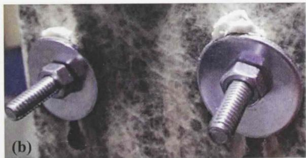
Figure 3.21: (a) Bending in the connecting bolts, (b) Folding of washers in W2\_D8\_ST\_1
