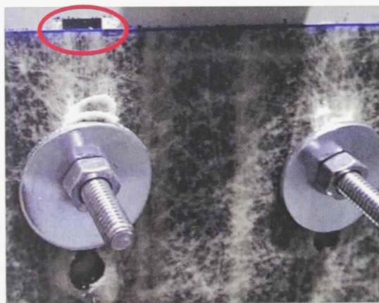
Figure 3.22: Initial tearing out failure in W2\_D8\_ST\_2
