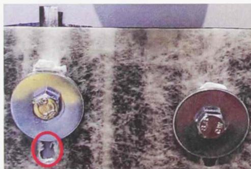
Figure 3.39: Rupture of the GFRP and CFRP in W2\_D6\_ST\_3 connection
