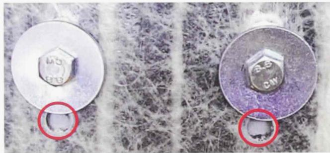
Figure 3.20: Bearing failure in W2\_D8\_ST\_2
