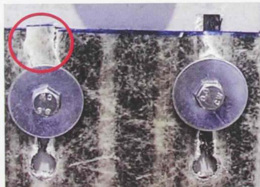
Figure 3.45: Block shear rupture of the HFRP laminates in W2\_D10\_ST\_2
