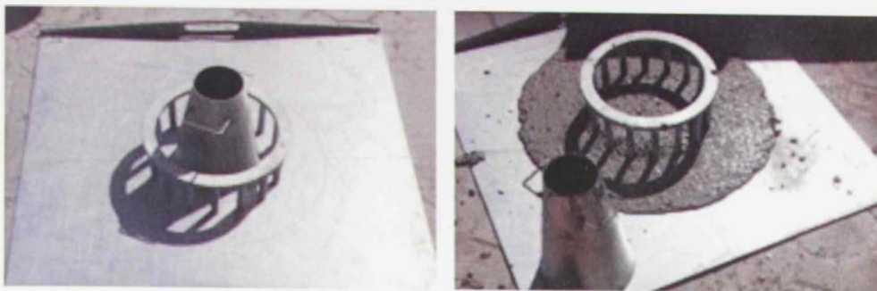
Figure 3-5: J-ring apparatus and test
