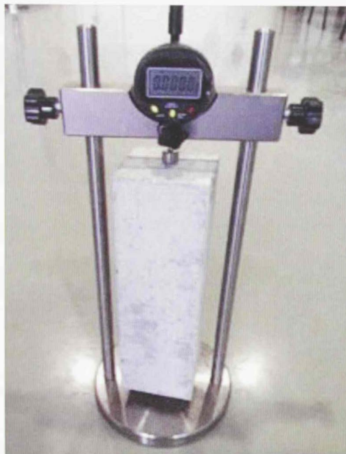
Figure 3-16: Drying shrinkage test setup
