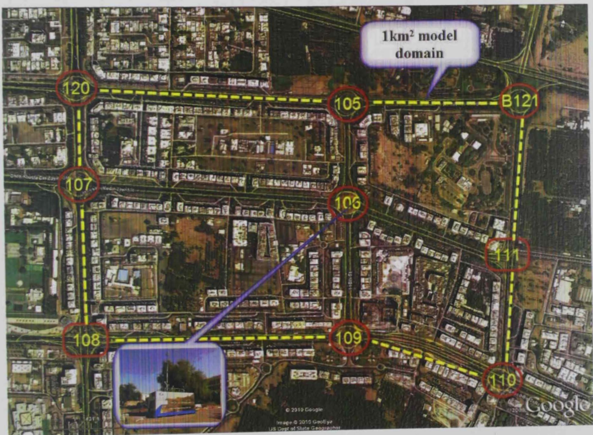
Fig. 6.18: The model domain used to determine pollutant concentration from vehicle traffic in the downtown area
