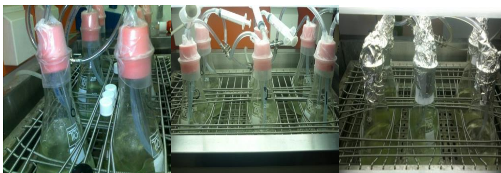
Figure A.2: Sides view of the 250 ml scale cultivation system
