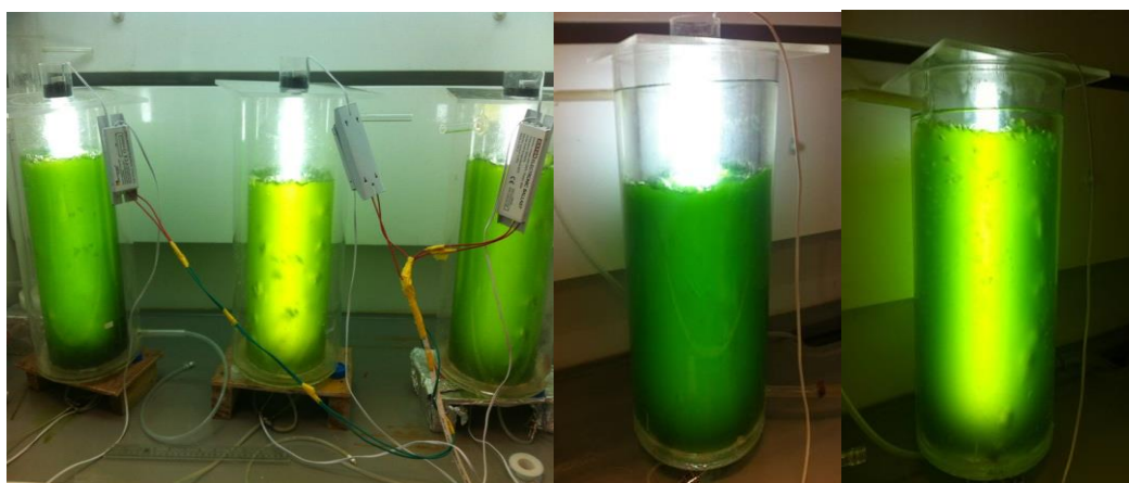
Figure A.3: Photographs on the 5 L photobioreactors with different culture densities
