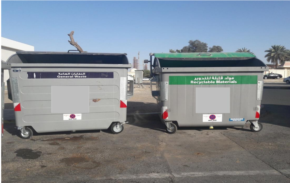
Figure A2: Bin size: 3 m 3 - Height: 1.54 m - Width: 2.02 m - Depth: 1.54 m
