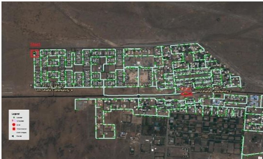
Figure 4.10: Optimal waste collection vehicle trip with relocation of waste bins based on a 40-m service zone
