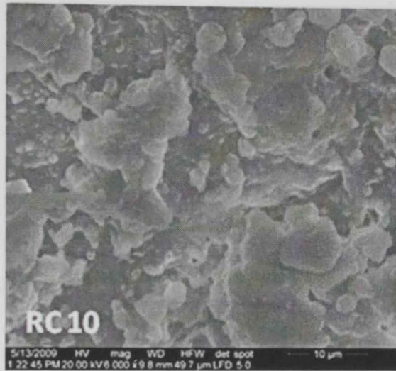
Figure 60. SEM micrographs of A) commercial 1, B) commercial 2, C) RC 10 membranes after filtration of 1000 ppm suspensions
