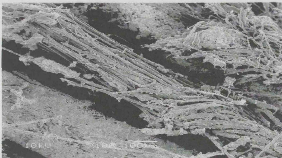
Figure 5.8: Layers cracking in the fractured immersed samples
