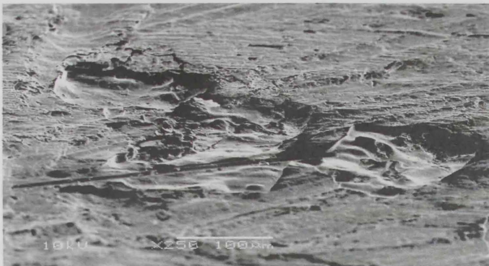
Figure 5.9: Leaching of the surface layer, hybrid composite
