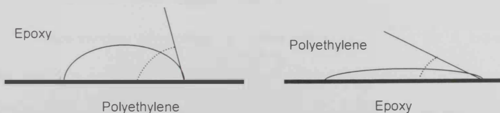
Fig 1.2 different behavior in spreading between Epoxy & Polyethylene
