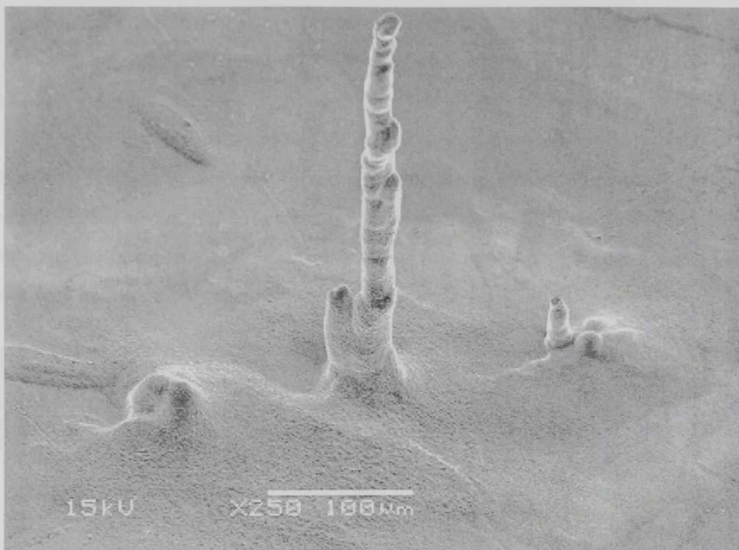
Figure 6.16-C: SEM image for a parallel deposition by using the heptode shown in figure 4.5. In this experiment not all of the heptode tips are active. Only 4 tips were activated. Actually the heptode was broken as the fiber containing the tips was very thin.
