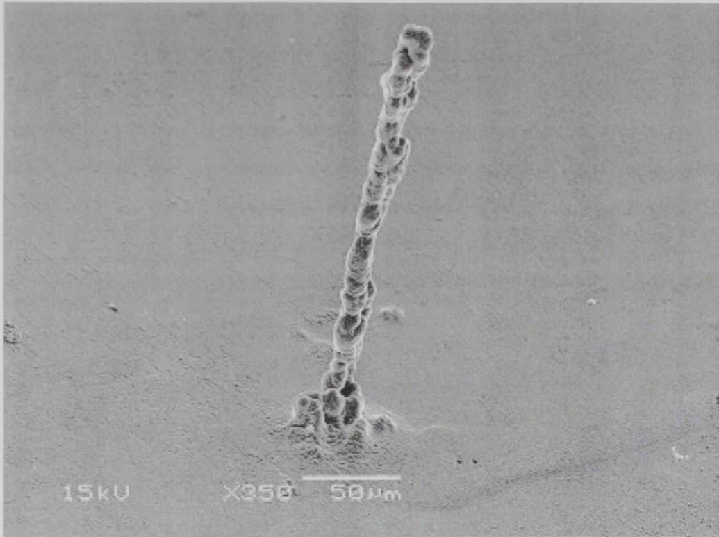
Figure 6.16-B: SEM image for a parallel deposition by using the heptode shown in figure 4.5. All of the 7 tips were activated. Due to the small distance between the array elements, mutual effect is taking place and the output structure is not 7 independent structures, rather, it is composed of a one-column structure. Note that the width is greater than the tip diameter that is around 7\mu\text{m} . These results agree with the simulation results presented earlier in chapter 5.
