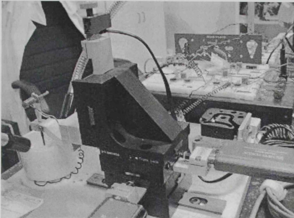
Figure 6.3: 3-D picomotors (from Newfocus Inc.) of resolution about 30nm per step is used to move the microelectrode array in the space. The movement of the picomotors is programmed by LabVIEW code according to the user requirements.
