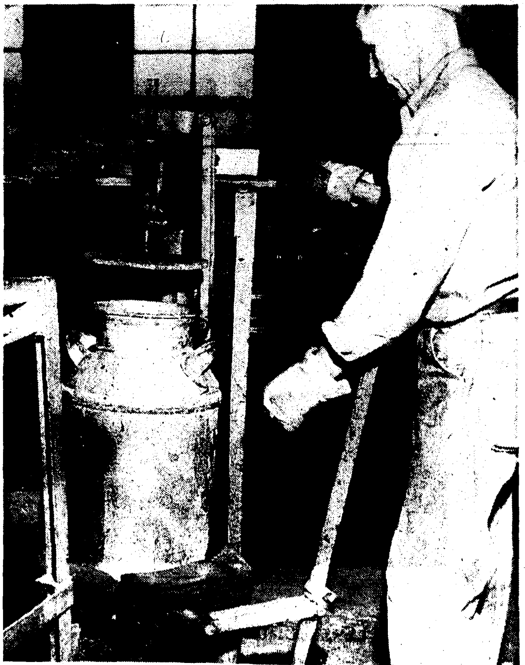
NEW BOTTOMS . . . Seamed cans which need new bottoms get them in this machine. Leonard Ellestad inserts the new bottom on the can and the machine crimps the edge to the cylinder.
