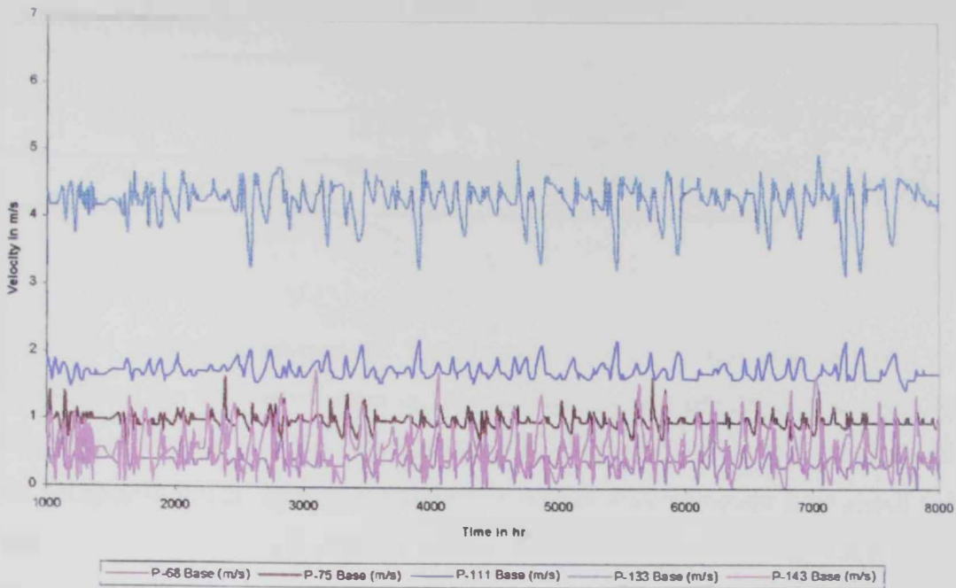
Figure 7.2 The pipes velocity of Al Yahar area accomplished with the proposed elevated tank at the entrance of the area
