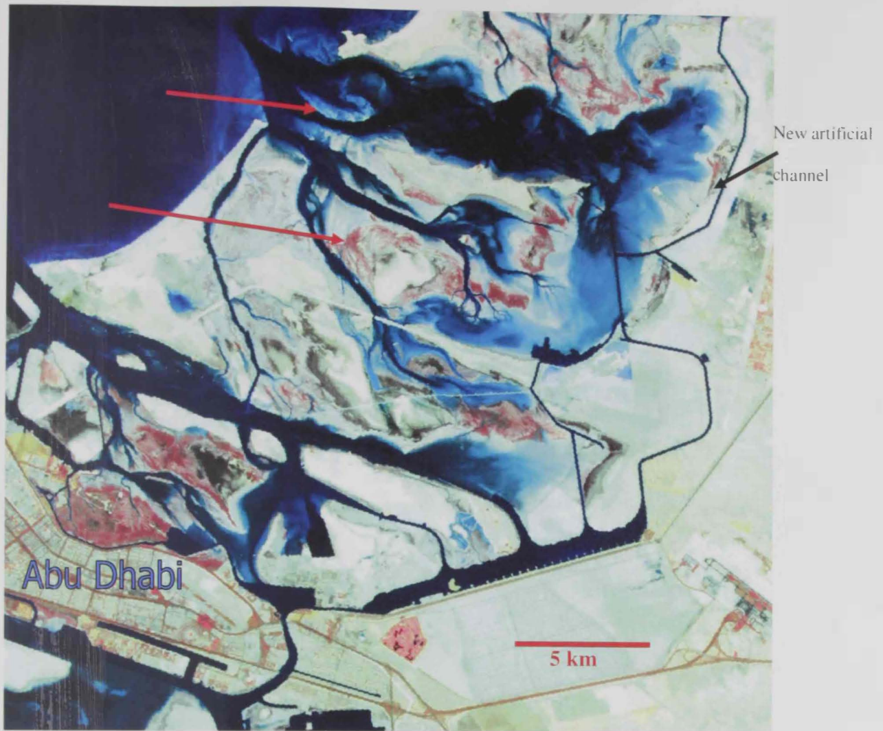
Figure 4-6: A Landsat –7 ETM satellite image of Abu Dhabi coastal zone area. Red arrows showing new islands appeared during the time 1993-2000.
