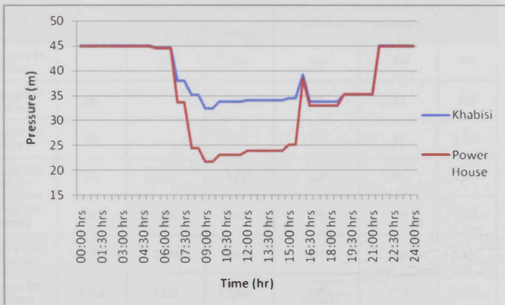
Figure 5.19: Residual pressure at Khabisi and Power House with C value of 100 except Power House branch (C=150)
