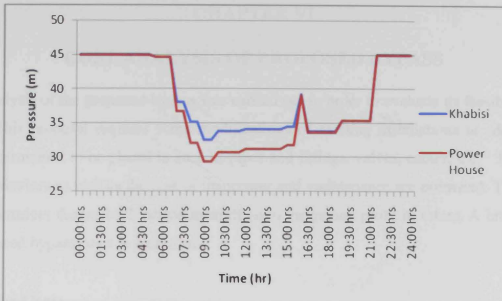
Figure 5.18: Residual pressures at Khabisi and Power House with C value of 100 and 900mm diameter Power House branch
