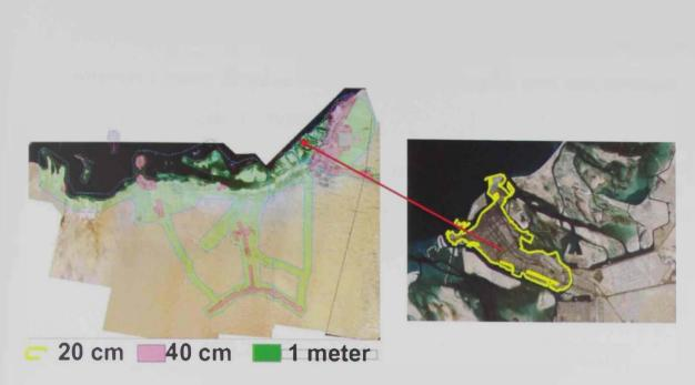
Fig. 4.3 Mapping Accuracy requirement in Abu Dhabi (Source: Abu Dhabi Municipality)
