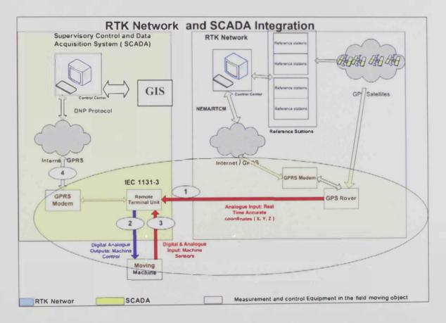
Fig. 8.1 Proposed RTK reference network & SCADA integration
