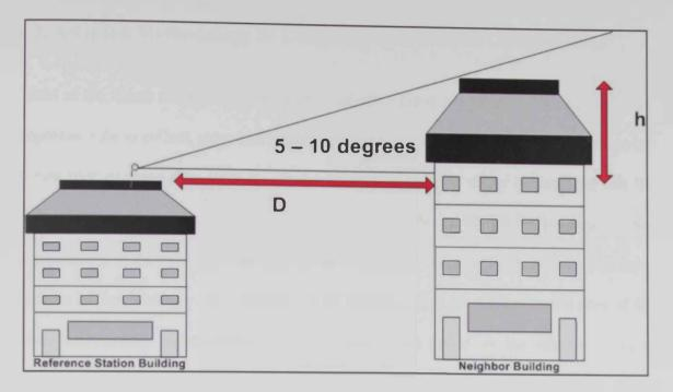
Fig. 6.2 Mask angle of the reference station's antenna
