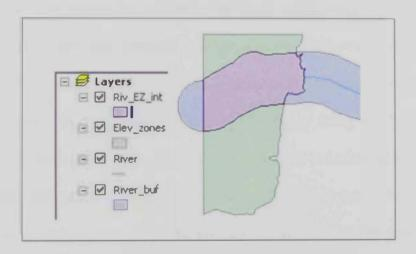
Fig. 2.4 An example of the buffer and overlay (intersect) tools.
