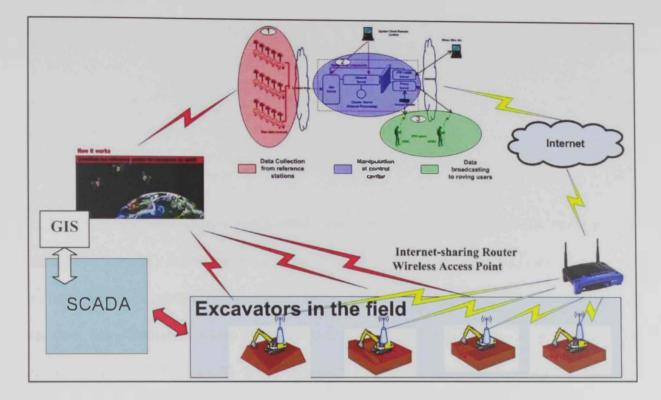
Fig. 8.3 The architecture of the proposed integrated system of RTK Network & SCADA/GIS for machine automation
