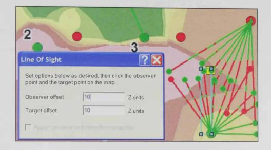
Fig. 7.3 Examining the line of sight between stations according to the observer and target heights from ground
