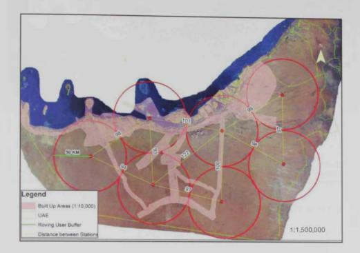
Fig. 5.3 Stations distribution based on user buffer of 50 km without overlap
