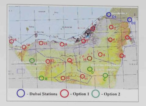
Fig. 4.2 Proposed distribution of the multi reference station in Abu Dhabi
