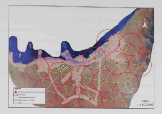
Fig. 5.1 Station Distribution based on user buffer of 35 km without overlap
