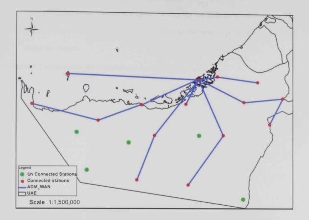
Fig. 7.1 Reference stations connectivity
