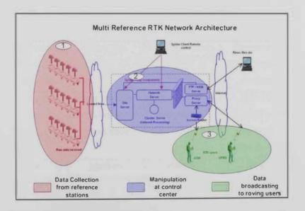
Fig. 3.4 RTK Reference Network architecture (Source: Lieca Geosystems)
