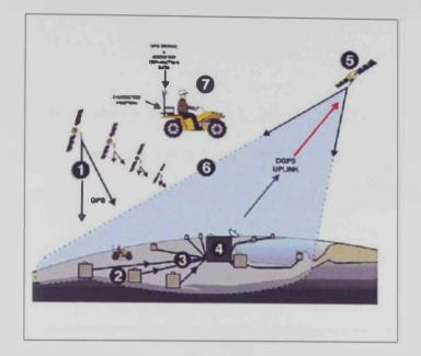
Fig. 3.2 SBAS Service Exemple : Omni STAR SBAS service
