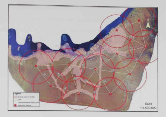
Fig. 5.4 Stations distribution based on user buffer of 50 km with overlap
