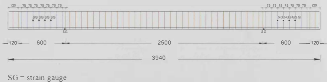
Figure 3.24: Positions of the strain gauges for specimens of group [C] (All dimensions are in mm)
