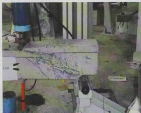
Figure 4.55: Failure mode of specimen D2-S2-NR
