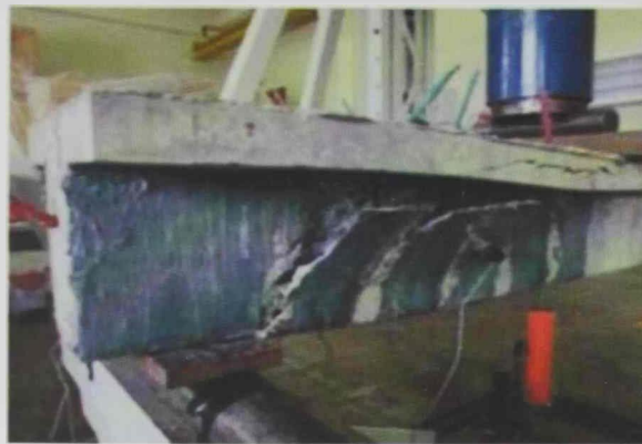
Figure 2.5: Detachment of the CFRP sheets failure mode at beam sides (El-Maaddawy and Chekfeh 2013)
