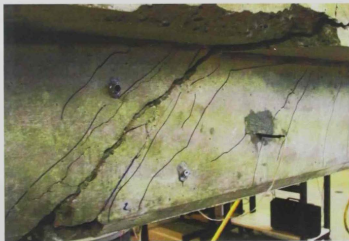
Figure 2.22: Diagonal tension shear mode of failure for the strengthened specimen (Mofidi et al. 2012)
