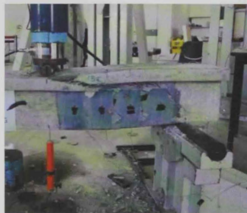
At failure (second shear test)
