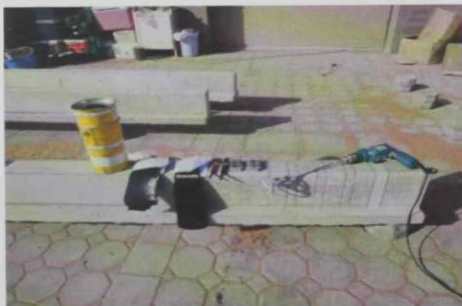
(a) Marked concrete after surface preparation
