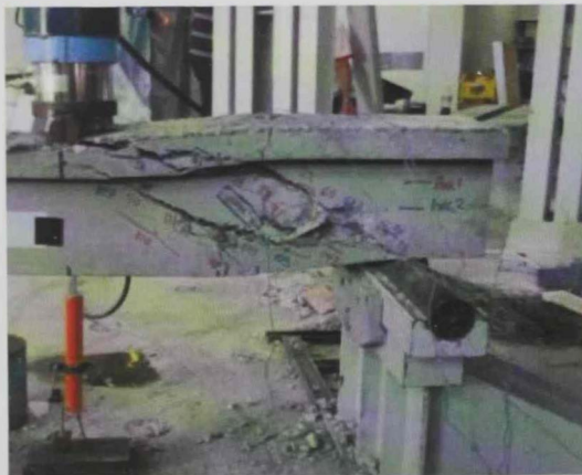
At failure (second shear test)
