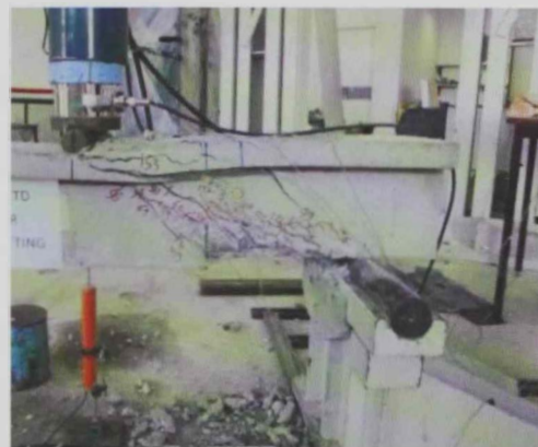
At failure (second shear test)
