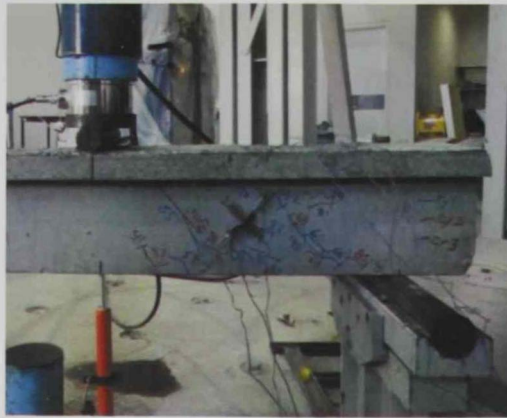
After initial shear damage D1
