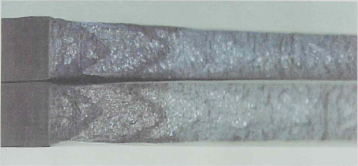
Figure 5.13 Sample photograph of crack front tunneling after crack initiation and maximum load in mixed mode.
