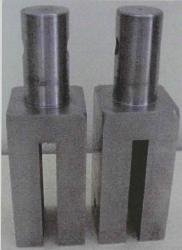
Figure 3.3 Photograph showing the fork-type fixture
