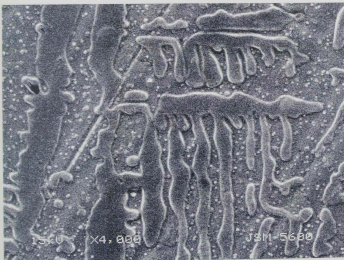
Figure III15a: SEM graph for SS 316 surface after oxide formation at E_{app.}(2) , t = 100 s .
